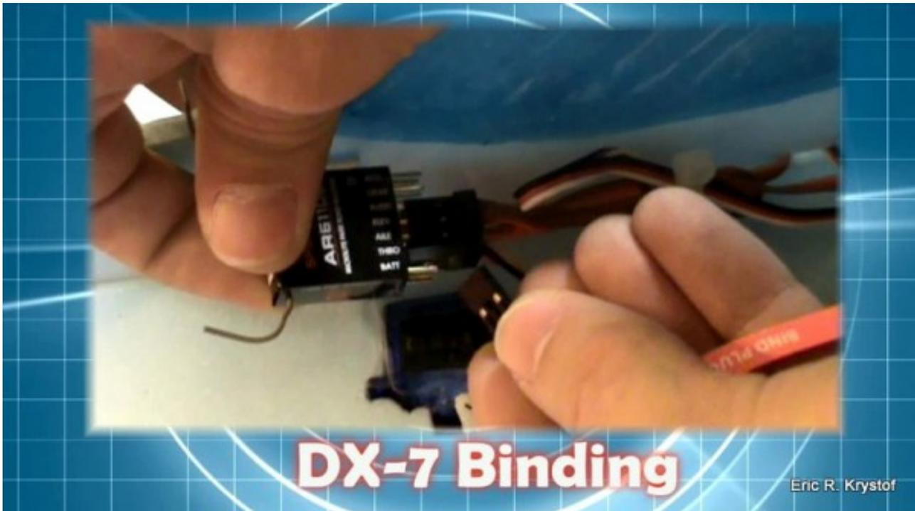
Inserting the bind plug into the BATT channel.
