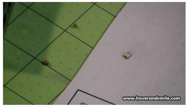
Third arms and alligator clips are just to big to easily handle these guys, so at this point I've used a small cardboard crade to hold these LEDs in. It's cheap, but it works. Just make sure you know which metal contact side is negative and positive, flip theLED over into the cradle, and get to putting some solder on the small metal contacts.
