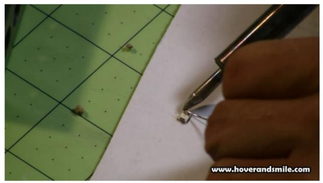
Of course, if you're really not sure which side is negative and which is positive, wire one up and put a 3V battery against it. It should be enough to light the LED and not kill it if you place the wrong voltage ends against it. Just don't do anymore than that, they're easily smoked.
