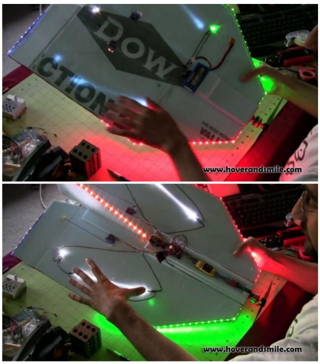
The designer of our combat flyer, Chameleon, has added a useful tip if you're looking to get some angled light effects on your plane, especially with the strip LEDs. A simple angled foam strip, with LEDs attached along the angle.
