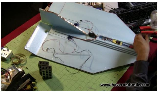
The SMD LEDs are simply strung through the middle of the fuselage to the underside, embedded similar to the bulb LEDs, and taped over with packing tape for protection.
